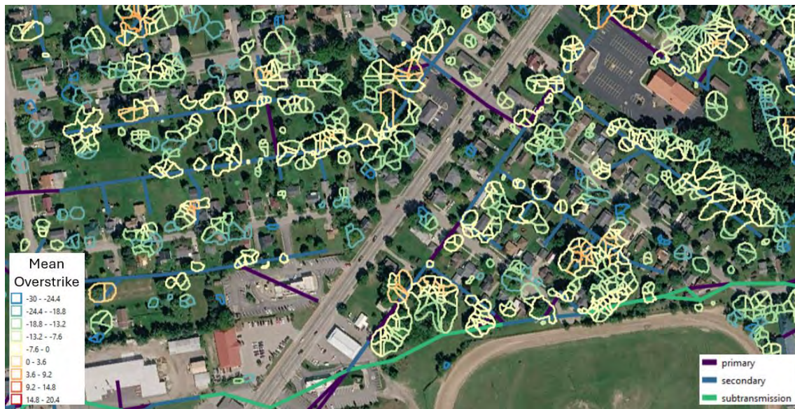
Figure B1. Illustration of canopy strike metric (canopy height - 3D distance to span). Negative numbers indicate tree heights too low to overstrike the conductor lines. Positive numbers indicate potential overstrike.
