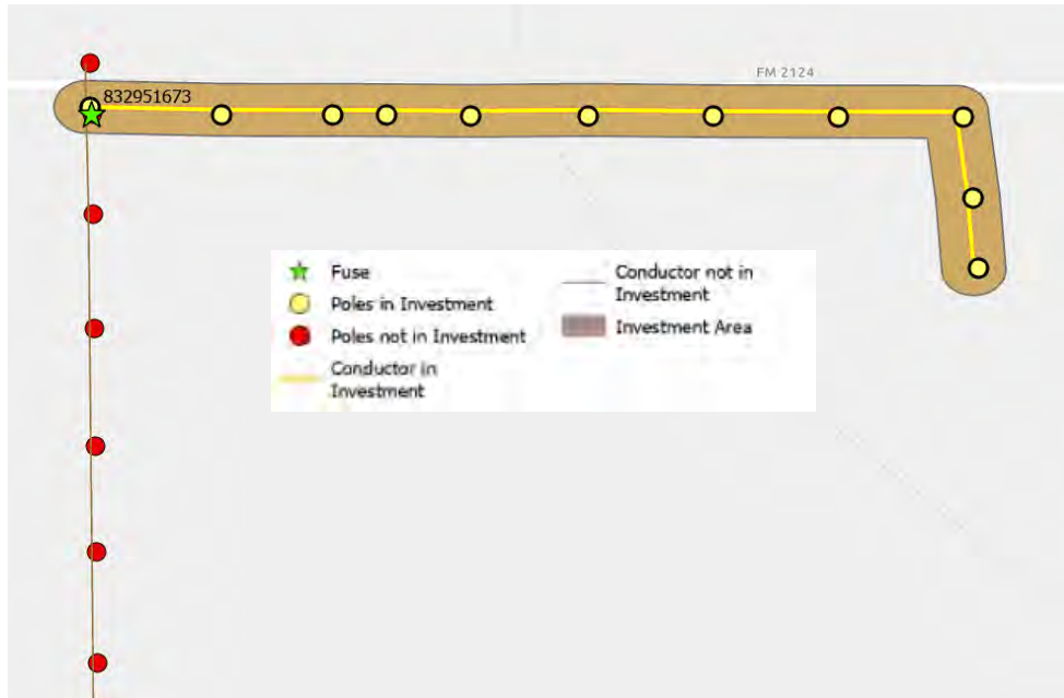
Figure 2-1: Asset to Protection Zone Relationship
