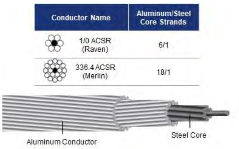
Exhibit 6.21 – ACSR Conductors for Small Wire Replacement
