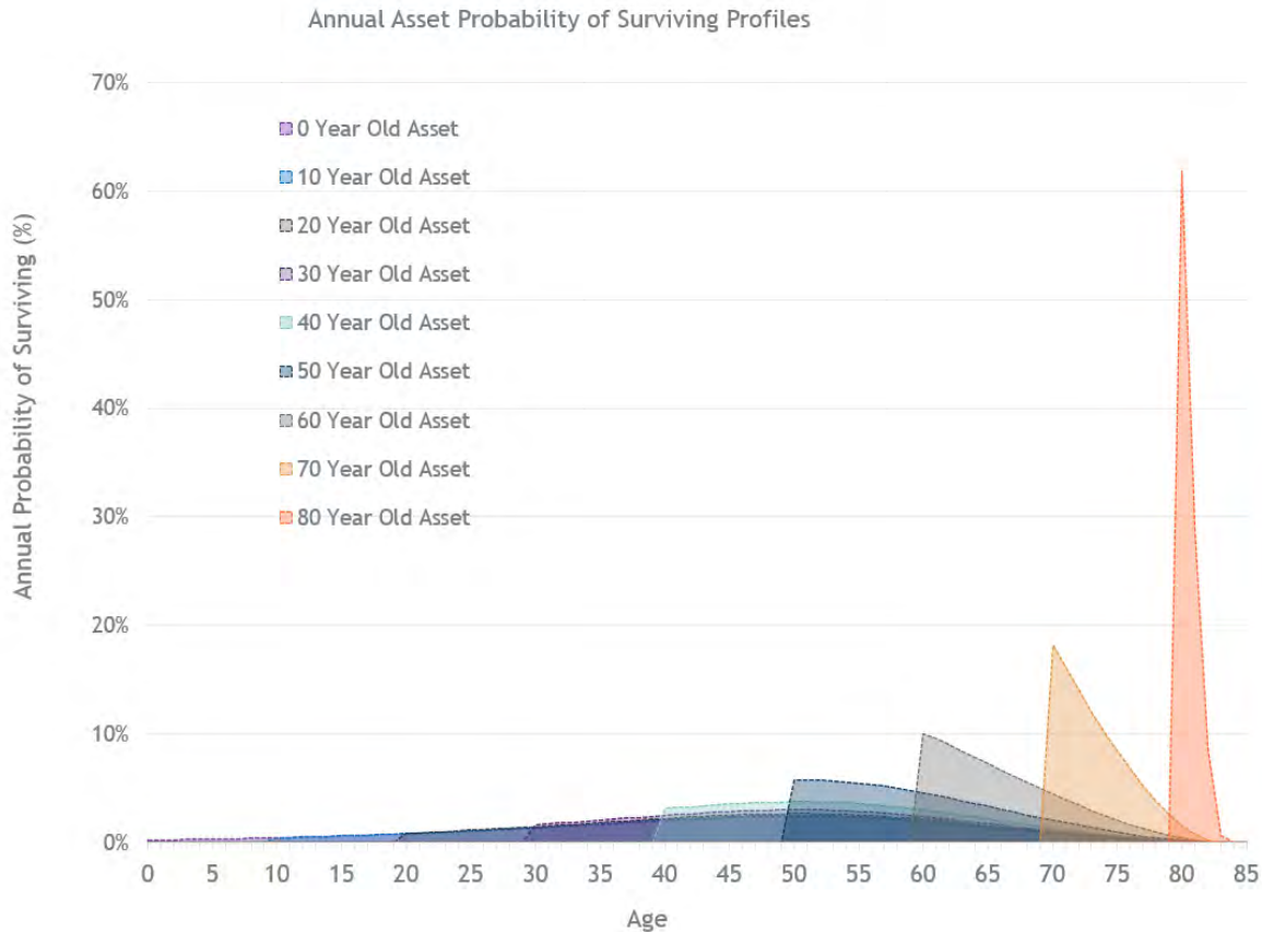
Figure 4-12: Survivor Curves to Annual Probability of Not Surviving Profiles for Oil Distribution Breakers
