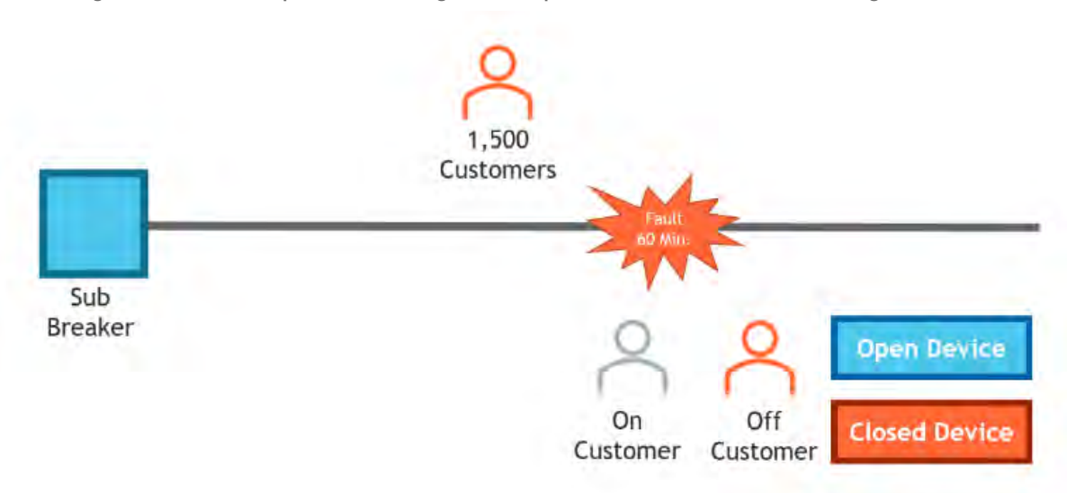
Figure 4-23: Simplified Outage Example without Sectionalizing Reclosers
